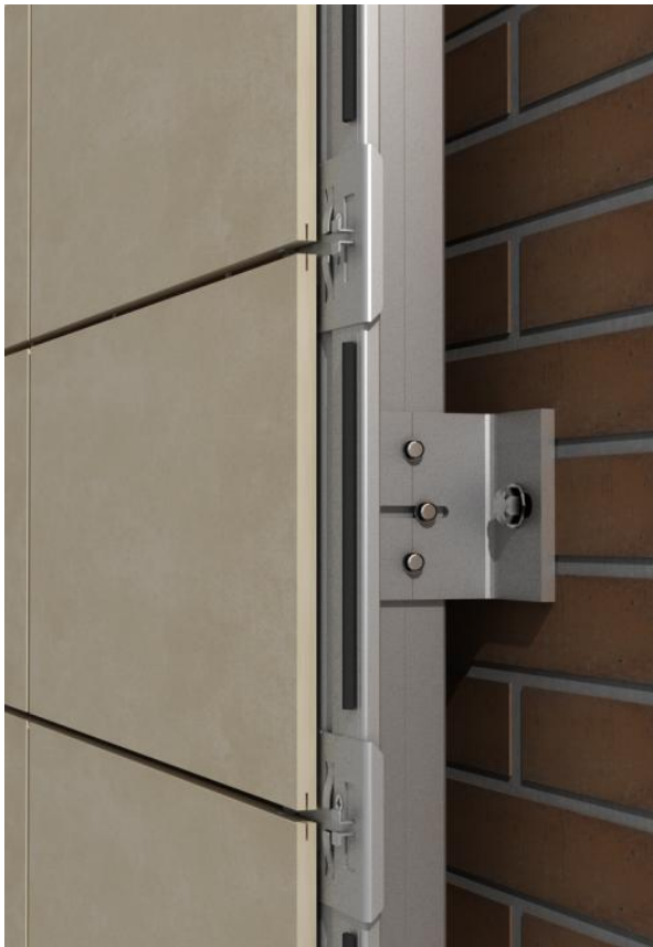
Figure A1.1: PF-ALT-SO assembled system.
